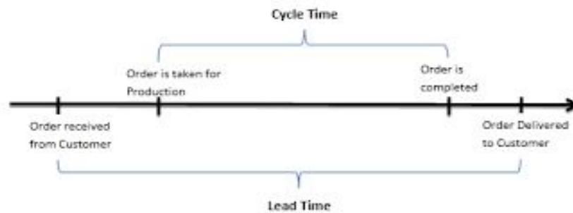
*Cycle Time*: Total time to complete production of one unit (work process based)
