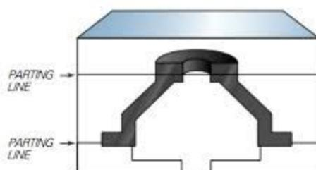
The parting line is the location on the part where the two halves of the mold meet for injection and split for ejection. This is where most flash is likely to occur from multiple factors like force from injection or an improper fit of the two halves. Flash at the parting line can be avoided by close inspection of the tool as well as investing in a high quality tool.
